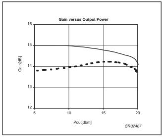
Figure 6. Gain vs. output power
